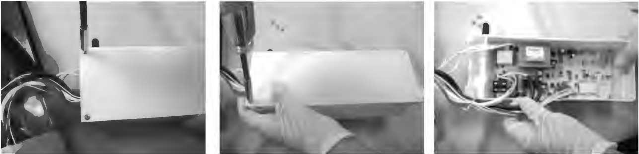
Picture 31 – 32 – 33 : Remove the 4 securing screws from the back of the box and lift off the cover.
