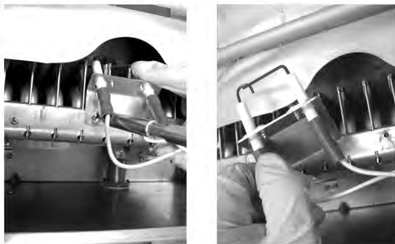
Picture 67 – 68 : The electrodes and earth cable assembly is removed by loosening the 2 securing screws using a star headed screwdriver.
