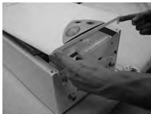
Picture 17 - 18: Remove the two screws from the bottom of the appliance as shown using a star head screw driver. Lift the front panel away from the appliance and push upwards to remove.
