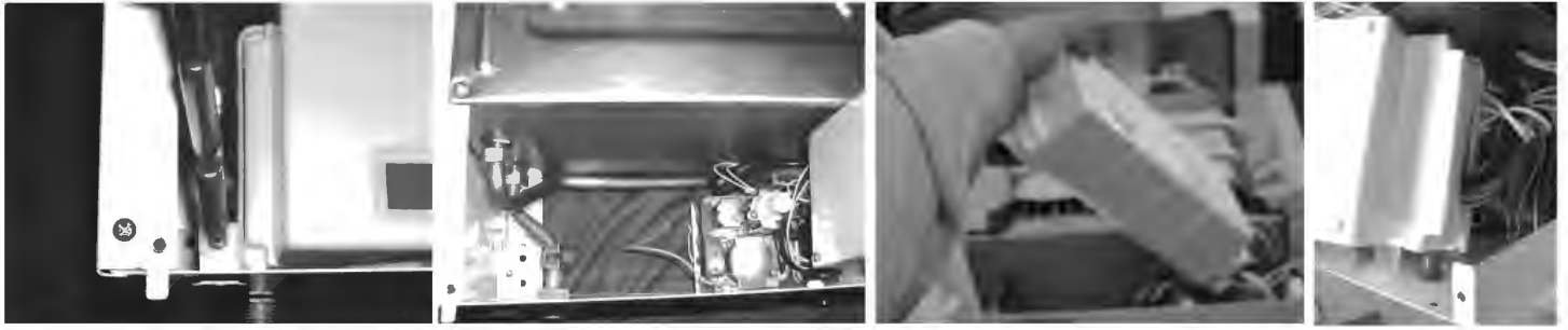
Picture 27 – 28 – 29 – 30 : Remove the two screws locating the control box and remove the box.
