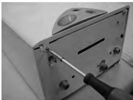
Picture 17 - 18: Remove the two screws from the bottom of the appliance as shown using a star head screw driver. Lift the front panel away from the appliance and push upwards to remove.
