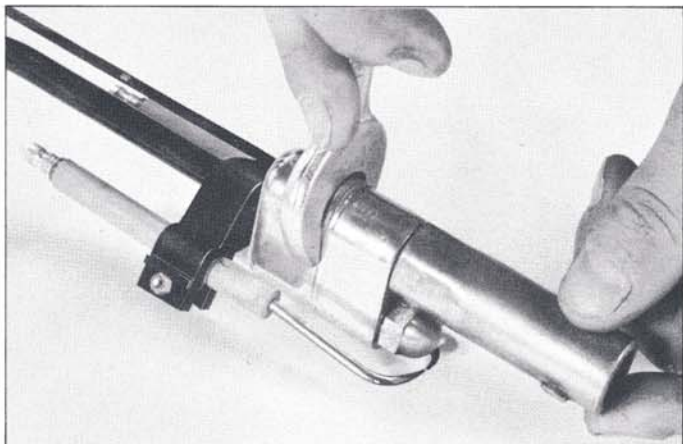
It is necessary to dismantle diffuser from inner assembly before nozzle removal. Nozzles are removed using a nozzle spanner. Fit nozzle to burner inner assembly by hand; use spanner only for final tightening. Re-assemble diffuser in correct position, i.e. diffuser retaining clamp firmly against nozzle shoulder or stop (see sketch).
