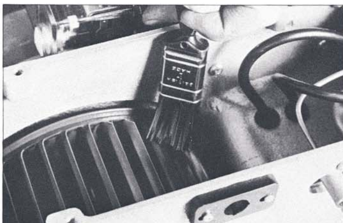
Cleaning the fan runner: use a stiff brush.
