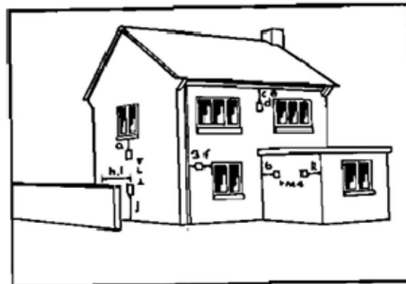
Fig.3 Netaheat flue terminal positions
