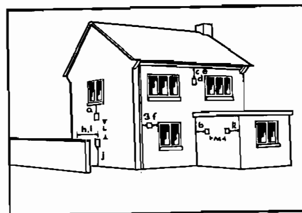
Fig.3 Netaheat flue terminal positions
